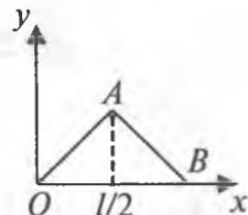
$$a_n = \frac{2}{l} \int_0^l f_1(x) \sin \frac{n\pi}{l} \cdot x dx = \frac{4h}{l^2} \int_0^{l/2} x \cdot \sin \frac{n\pi}{l} \cdot x dx + \frac{4h}{l^2} \int_{l/2}^l (l-x) \cdot \sin \frac{n\pi}{l} \cdot x dx.$$
