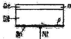
III.61-rasm. Epitaksial p - n o'tish.
