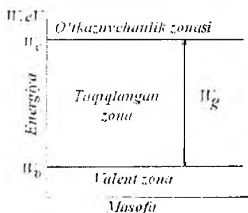
1.2-rasm. Qattiq jism zonalar energetik diagrammasi.
