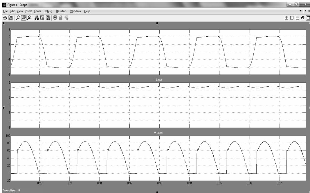
11-rasm. Yuklamadagi kuchlanish va yuklama, ta'minotdagi tok ossillogrammasi
