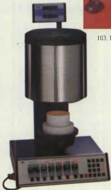
104. Keramikani havoda kuydiruvchi pechka (VITA VACUMAT).
