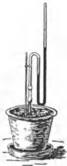
15- rasm. Simob manometri vositasida suv tomchilash bosimini o'lchash.
