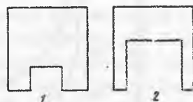
38-rasm. PPU-3N penoplastining zararlanish intensivligi: Plastinka tishli kalamush (2). Kulrang kalamush (1) (24 soatlik tajribada) (I.A.Yemelyanova bo'yicha, 1978).
