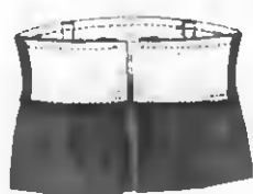
59-rasm. Belbog' bilan yaxlit bichilgan yubka yuqori chetiga ishlov berish:
