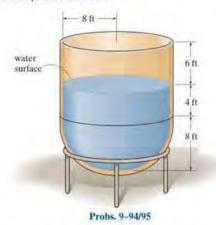
\*9-96. Determine the surface area of the tank, which consists of a cylinder and hemispherical cap.
