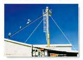
If an x, y, z coordinate system is established, then the coordinates of points A and B can be determinded. From this the position vector  $\mathbf{r}$  acting along the cable can be formulated. Its magnitude represents the length of the cable, and its unit vector,  $\mathbf{u} = \mathbf{r}/r$ , gives the direction defined by  $\alpha$ ,  $\beta$ ,  $\gamma$ .
