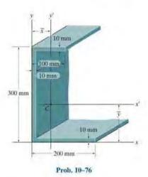
•10-77. Determine the product of inertia of the beam's cross-sectional area with respect to the centroidal x and
