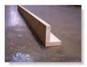
The effectiveness of this beam to resist bending can be determined once its moments of inertia and its product of inertia are known.
