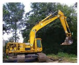
P6-3. Draw the free-body diagrams of the boom ABCDF and the stick FGH of the bucket lift. Neglect the weights of the member. The bucket weighs W. The two force members are BI, CE, DE and GE. Assume all indicated points of connection are pins.
