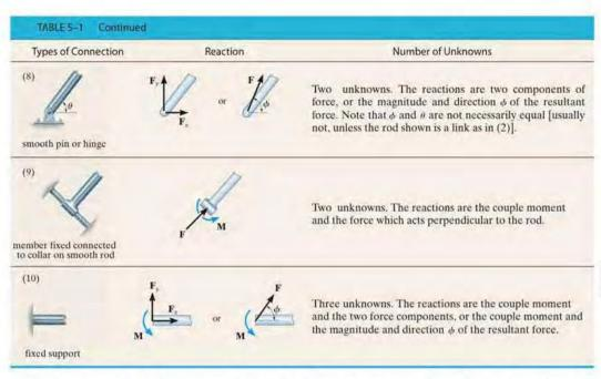
Typical examples of actual supports are shown in the following sequence of photos. The numbers refer to the connection types in Table 5-1.
