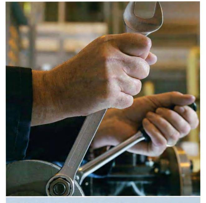
Application of forces to the handles of these wrenches will produce a tendency to rotate each wrench about its end. It is important to know how to calculate this effect and, in some cases, to be able to simplify this system to its resultants.
