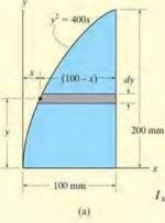
Determine the moment of inertia for the shaded area shown in Fig. 10-6a about the x axis.
