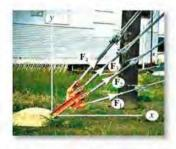
The resultant force of the four cable forces acting on the supporting bracket can be determined by adding algebraically the separate x and y components of each cable force. This resultant F<sub>R</sub> produces the same pulling effect on the bracket as all four cables.
