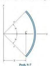
**\*9–8.** Determine the area and the centroid  $(\bar{x}, \bar{y})$  of the area.
