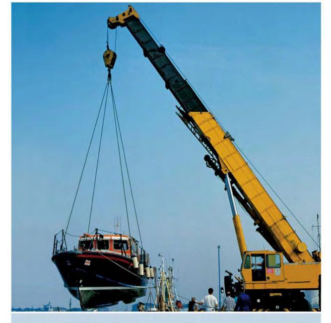
The crane is subjected to its weight and the load it supports. In order to calculate the support reactions on the crane, it is necessary to apply the principles of equilibrium.
