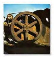
This flywheel, which operates a metal cutter, has a large moment of inertia about its center. Once it begins rotating it is difficult to stop it and therefore a uniform motion can be effectively transferred to the cutting blade.
