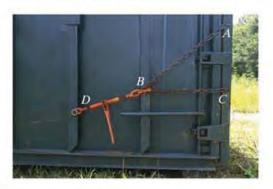
P3-4. The two chains AB and AC have equal lengths and are subjected to the vertical force F. If AB is replaced by a shorter chain AB', show that this chain would have to support a larger tensile force than AB in order to maintain equilibrium.
