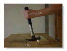
The ability to remove the nail will require the moment of  $\mathbf{F}_H$  about point O to be larger than the moment of the force  $\mathbf{F}_N$  about O that is needed to pull the nail out.
