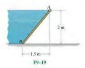
**F9–20.** Determine the magnitude of the hydrostatic force acting on gate AB, which has a width of 2 m. Water has a density of  $\rho = 1 \text{ Mg/m}^3$ .
