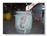
The moment of the applied force  $\mathbf{F}$  about point O is easy to determine if we use the principle of moments. It is simply  $M_O = F_x d$ .
