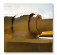
This thrust bearing is used to support the drive shaft on a machine. (7)
