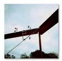
The projection of the cable force  $\mathbf{F}$  along the beam can be determined by first finding the unit vector  $\mathbf{u}_h$  that defines this direction. Then apply the dot product,  $F_h = \mathbf{F} \cdot \mathbf{u}_h$ .
