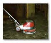
The motor that turns the disk of this sanding machine develops a torque that must overcome the frictional forces acting on the disk.
