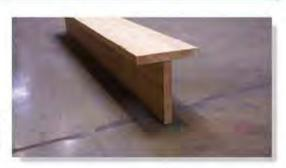
For design or analysis of this Tee beam, engineers must be able to locate the centroid of its cross-sectional area, and then find the moment of inertia of this area about the centroidal axis.
