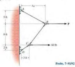
•7–93. Determine the force P needed to hold the cable in the position shown, i.e., so segment BC remains horizontal. Also, compute the sag  $y_B$  and the maximum tension in the cable.
