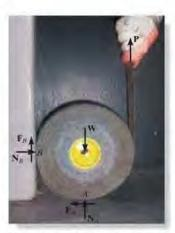
The applied vertical force P on this roll must be large enough to overcome the resistance of friction at the contacting surfaces A and B in order to cause rotation.
