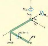
Moment components are developed by the pin on the rod to prevent rotation about the x and z axes.
