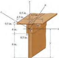
\*10-80. Locate the centroid  $\bar{x}$  and  $\bar{y}$  of the cross-sectional area and then determine the orientation of the principal axes, which have their origin at the centroid C of the area. Also, find the principal moments of inertia.
