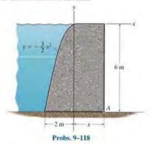
9-119. The underwater tunnel in the aquatic center is fabricated from a transparent polycarbonate material formed in the shape of a parabola. Determine the magnitude of the hydrostatic force that acts per meter length along the surface AB of the tunnel. The density of the water is  $\rho_n = 1000 \text{ kg/m}^3$ .
