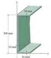
10-75. Locate the centroid  $\vec{x}$  of the beam's cross-sectional area and then determine the moments of inertia and the product of inertia of this area with respect to the u and v axes. The axes have their origin at the centroid C.
