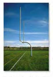
Integration must be used to determine the location of the center of gravity of this goal post due to the curvature of the supporting member.
