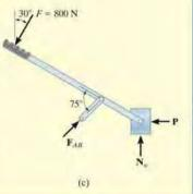
Before proceeding, it is highly recommended that you cover the solutions to the previous examples and attempt to draw the requested free-body diagrams. When doing so, make sure the work is neat and that all the forces and couple moments are properly labeled. When finished, challenge yourself and solve the following four problems.
