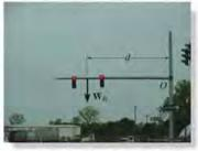
Here the weights of the traffic lights are replaced by their resultant force  $W_R = W_1 + W_2$ which acts at a distance  $d = (W_1d_1 + W_2d_2)/W_R$  from O. Both systems are equivalent.
