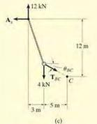
Since the sag  $y_C = 12$  m is known, we will now consider the leftmost section, which cuts cable BC, Fig. 7–19c,
