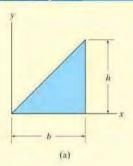
Determine the product of inertia  $I_{xy}$  for the triangle shown in Fig. 10-14a.
