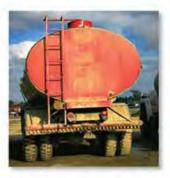
The resultant force of the water pressure and its location on the elliptical back plate of this tank truck must be determined by integration.
