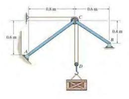
•6-129. Determine the force in each member of the truss and state if the members are in tension or compression.
