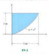
F9-2. Determine the centroid  $(\bar{x}, \bar{y})$  of the shaded area.
