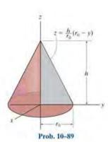
**10–90.** Determine the mass moment of inertia  $I_x$  of the right circular cone and express the result in terms of the total mass m of the cone. The cone has a constant density  $\rho$ .
