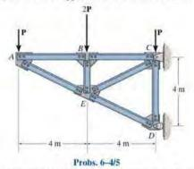
**6-6.** Determine the force in each member of the truss and state if the members are in tension or compression. Set  $P_1 = 2 \text{ kN}$  and  $P_2 = 1.5 \text{ kN}$ .
