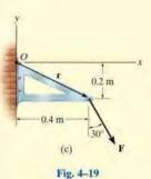
Force **F** acts at the end of the angle bracket shown in Fig. 4–19a, Determine the moment of the force about point O.
