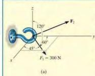
Two forces act on the hook shown in Fig. 2–32a. Specify the magnitude of  $\mathbf{F}_2$  and its coordinate direction angles of  $\mathbf{F}_2$  that the resultant force  $\mathbf{F}_R$  acts along the positive y axis and has a magnitude of 800 N.
