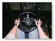
Steering wheels on vehicles have been made smaller than on older vehicles because power steering does not require the driver to apply a large couple moment to the rim of the wheel.
