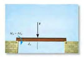
As illustrated by the example problems, the moment of a force does not always cause a rotation. For example, the force  $\mathbf{F}$  tends to rotate the beam clockwise about its support at A with a moment  $M_A = Fd_A$ . The actual rotation would occur if the support at B were removed.
