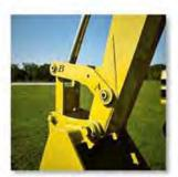
The bucket link AB on the back-hoe is a typical example of a two-force member since it is pin connected at its ends and, provided its weight is neglected, no other force acts on this member.
