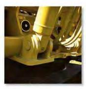
This pin is used to support the end of the strut used on a tractor. (8)
