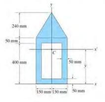
•10–49. Determine the moment of inertia  $I_{s'}$  of the section. The origin of coordinates is at the centroid C.
