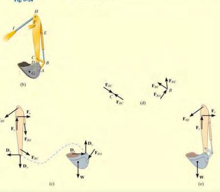
Draw the free-body diagram of each part of the smooth piston and link mechanism used to crush recycled cans, which is shown in Fig. 6–25a.
