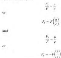
Here the y component is a negative scalar since  $\mathbf{F}_y$  is directed along the negative y axis.
