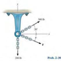
2-31. Three cables pull on the pipe such that they create a resultant force having a magnitude of 900 lb. If two of the cables are subjected to known forces, as shown in the figure, determine the angle  $\theta$  of the third cable so that the magnitude of force F in this cable is a minimum. All forces lie in the x-y plane. What is the magnitude of F? Hint: First find the resultant of the two known forces.
