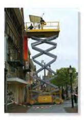
This scissors lift has one degree of freedom. Without the need for dismembering the mechanism, the force in the hydraulic cylinder AB required to provide the lift can be determined directly by using the principle of virtual work.
