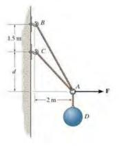
\*3-20. Determine the tension developed in each wire used to support the 50-kg chandelier.
