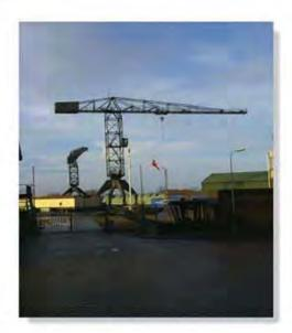
Simple trusses are often used in the construction of large cranes in order to reduce the weight of the boom and tower.
