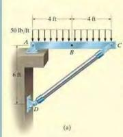
Determine the normal force, shear force, and bending moment acting at point B of the two-member frame shown in Fig. 7-6a.
