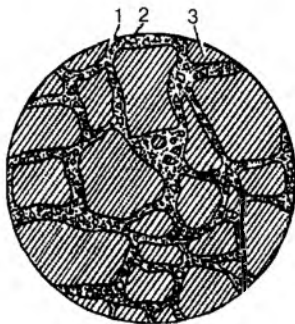
69-rasm. Odatdagi og'ir beton tuzilishining chizmasi:
