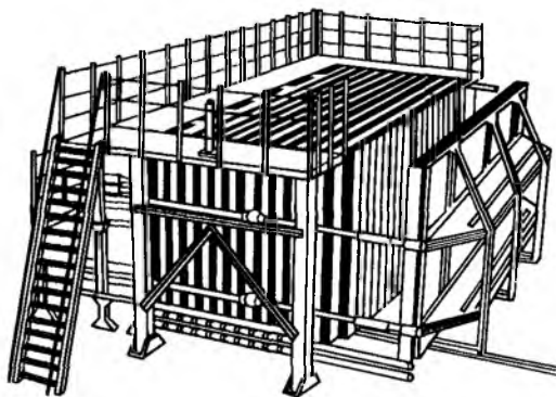
90-rasm. Temir-beton panellar tayyorlanadigan universal kasseta.
