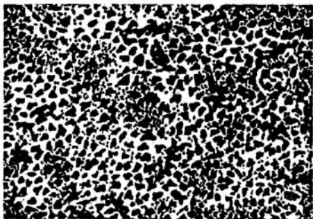
77-rasm. G'ovak beton tuzilishi.
