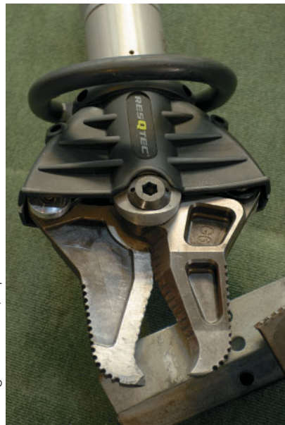
This "jaws-of-life" machine is used by rescuers to pry apart wreckage.
