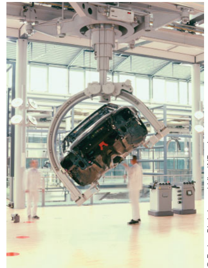
This apparatus is designed to hold a car body in equilibrium for a wide range of orientations during vehicle production.
