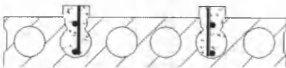
2.14-rasm. Ko'p bo'shliqli orayopma yoki tomyopma plitani kuchaytirish.
