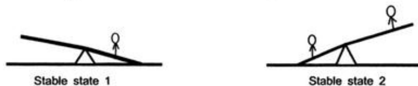
FIG. 6.1 A seesaw in one of the two stable states.
