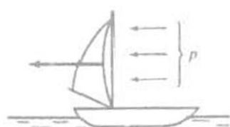
1.5-rasm. Shamolning dinamik bosimidan elkan yordamida harakatni yuzaga keltirishda foydalanish
