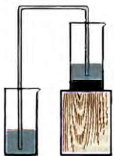
9-rasm. Loyqa suvni stakanda tindirish va undan toza tiniq suvni ajratib olish.
