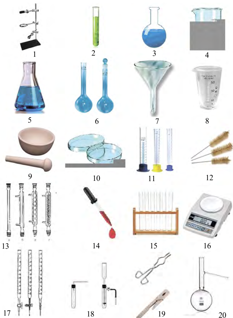
4-rasm. 1–universal shtativ; 2–probirka; 3–tubi yumaloq kolba; 4–o‘lchov stakani; 5–konussimon kolba; 6–o‘lchov kolbalari; 7–chinni voronkalar; 8–menzurka; 9–chinni hovoncha va dastasi; 10–Petri idishi; 11–o‘lchov silindrlari; 12–probirka tozalagich; 13–sovitkich; 14–pipetka; 15–probirka qo‘ygich; 16–elektron tarozi; 17–byuretkalar; 18–gaz olish asbobi; 19–qisqichlar; 20–Vyurs kolbasi.
