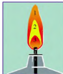
5-rasm. Spirt lampasi alangasining tuzilishi.
