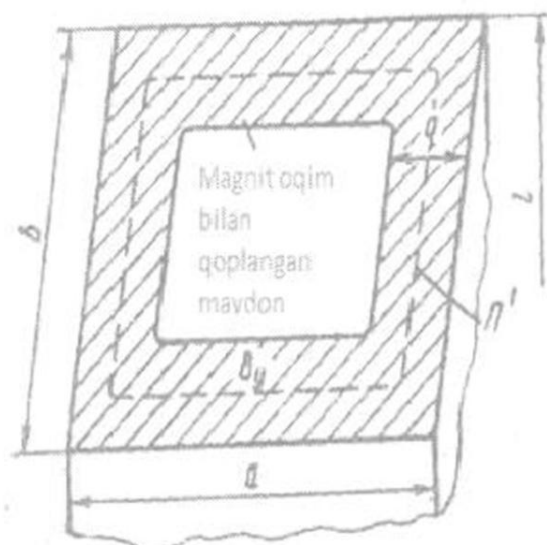
5.4-rasm. Magnit o'zakka magnit oqimining singishini tushuntirish uchun.
