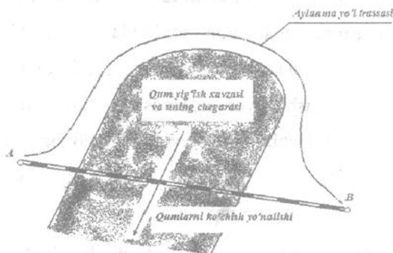
5.13 - rasm. Ko'chki qumli cho'llarda temir yo'llarni trassalash
