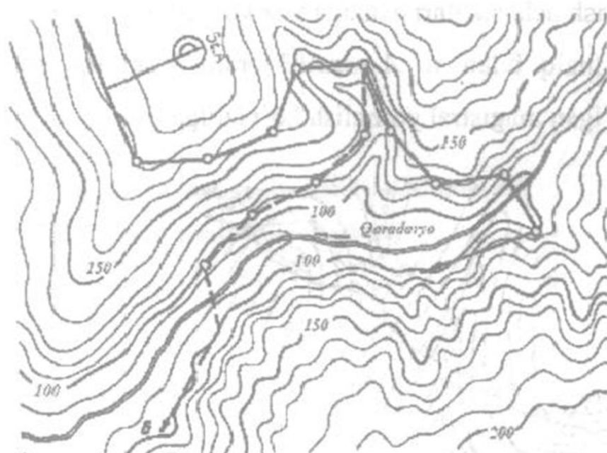
5.18-rasm. Zo'riqib yurish uchastkasining holatini trassa uzunligiga ta'siri
