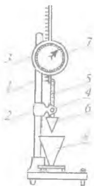
8.1-rasm Qorishma aralashmasining harakatchanligini aniqlash uchun standart konus asbobi:
