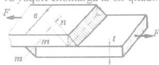
4.13-rasm. Ustma-ust payvandlash.
