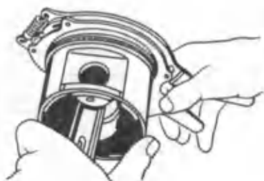
2.49-rasm. Ajratkich yordamida porshendan porshen halqalarini ajratib olish.
