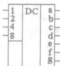
9.12-rasm. Yetti segmentlik indikatorning ko'rinishi va segmentlari nomi (a) hamda shartli-grafik belgilanishi (b).
