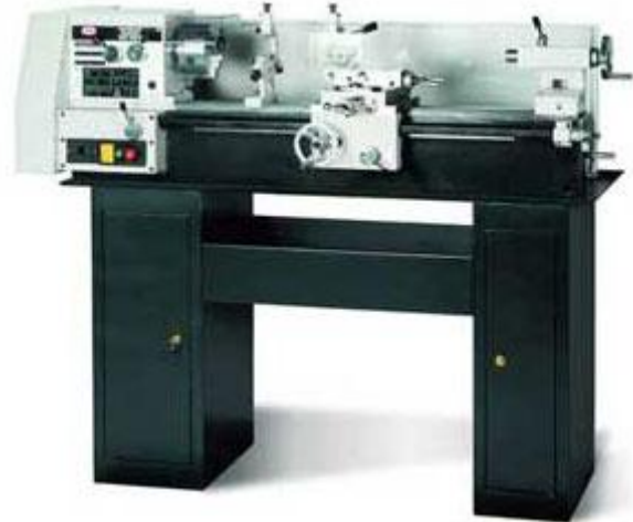
5.20--rasm. Universal tokarlik stanogi SPA-700P
