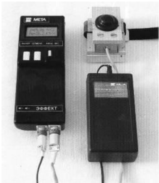
4.3-rasm. Tormoz tizimining samaradorligini aniqlovchi Effekt-02 jihozi
