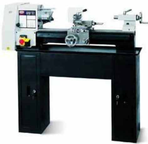
5.19--rasm. Universal tokarlik stanogi SPA-500
