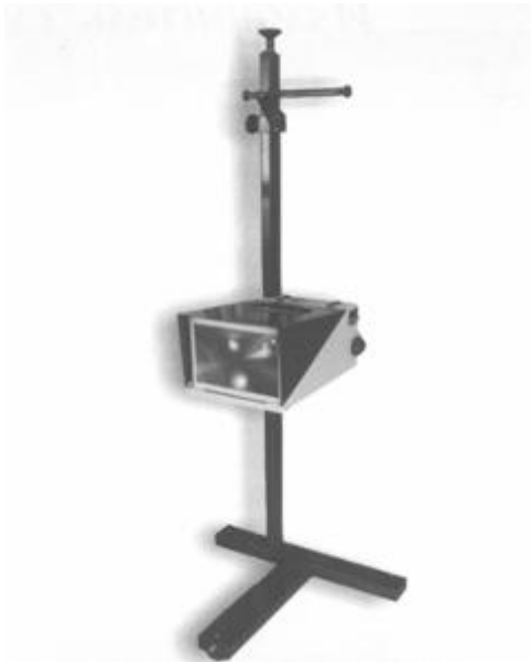
4.10-rasm. Avtomobil faralarining parametrlarini diagnostikalash uchun IPF-01 jihozi (a) va tekshirish jarayoni (b)
