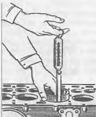
55-rasm. Porshen va silindr orasidagi tirgishni tekshirish shakli
