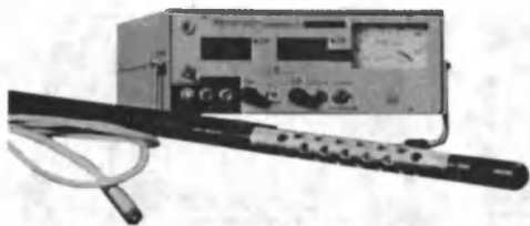
2.31-rasm. Avtotest-01.04 rusumli gazoanalizator-tutino'Ichagich (SO, SN, ayl/min, tutash darajasini o'lchaydi; 0-10 % SO, 0-5000 ppm CH, 0-10000 ayl/min, 0-10 m 1 / 0-100 % tutash darajasi; elektr iste'moli 12 va 220 V; tashqi o'lchamlari 290x98x300 mm; og'irligi 4,3 kg).
