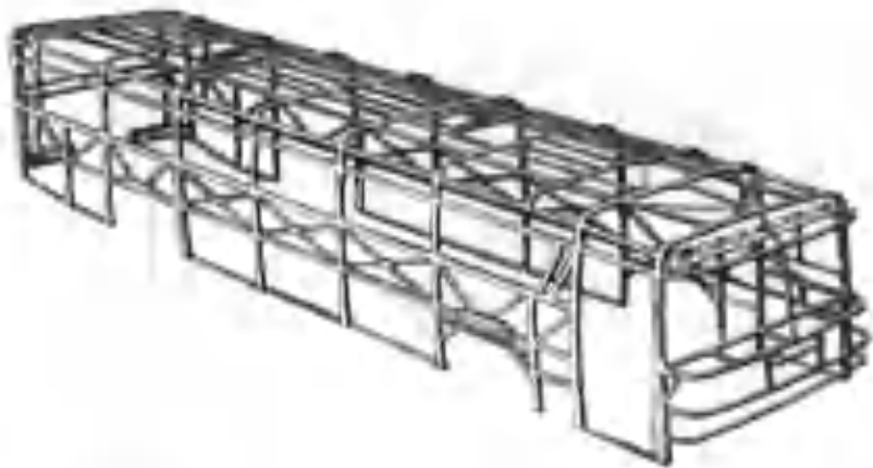
2.10-rasm. Mercedes katta shahar avtobusining kuzov karkasi.
