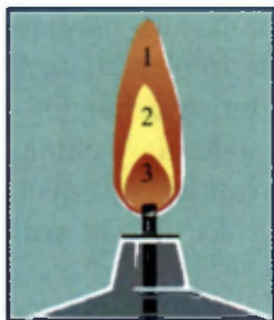
5-rasm. Spirt lampasi alangasining tuzilishi.
